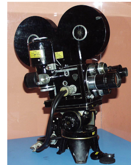
Figure 1.42 A specially constructed high-speed, high-quality movie camera to film nuclear explosions (Bradbury Museum, Los Alamos)
